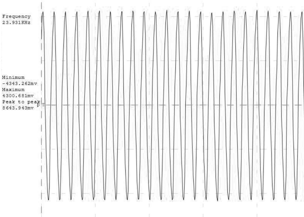
Figure 18: Expected waveform at C2 output when the circuit is correctly tuned.
