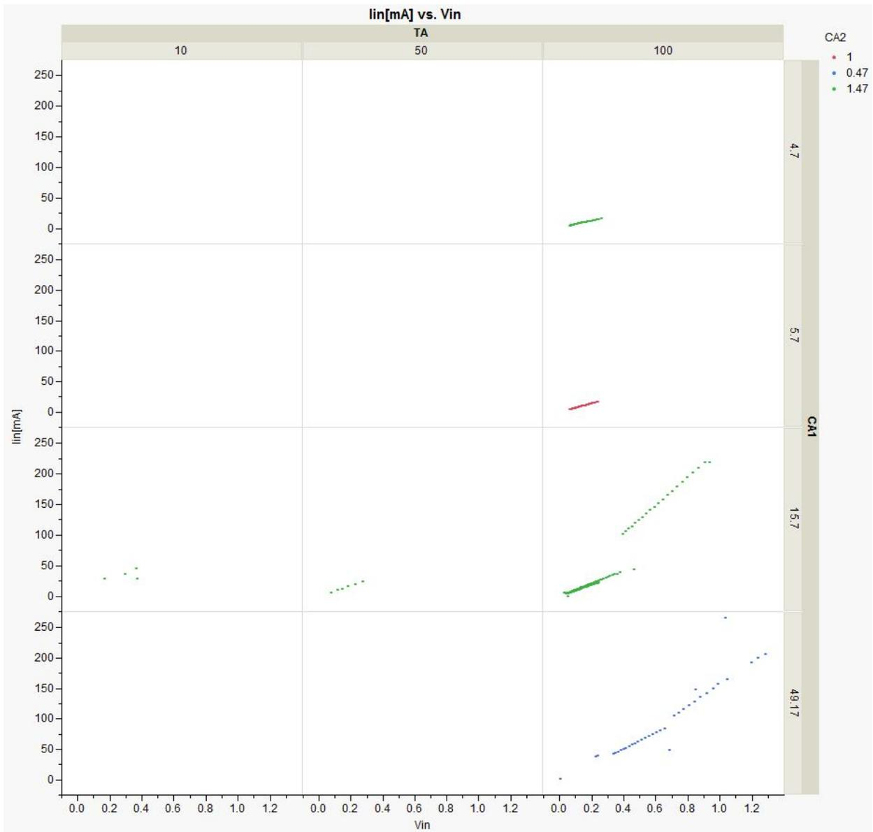
Figure 33: Input current / input voltage characterization as a function of turns ratio (TA) and capacitor values (CA1, CA2).
