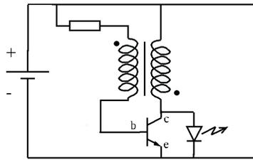
What a Joule Thief cannot do is operate with very low voltage and current sources. It generally needs input voltages that exceed 0.75 volts. The relatively low efficiency of the circuit may also become an issue. We note that zero threshold transistors [2] might be a way to get around some limitation, but design and results are still under development.
