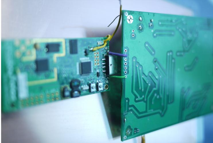
Figure 29: Telos B connected to PowerMod. Bottom view. Top view can be seen in Figure 24.
