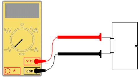
Figure 25: Measure Voltage
