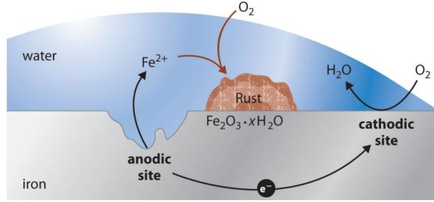
Figure 1: Illustration of the creation of rust
