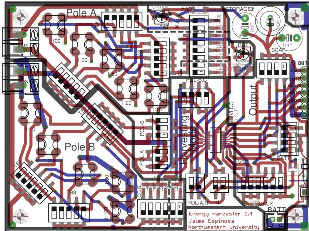
Figure 31: PCB layout of PowerMod. The ground plane is not shown.
